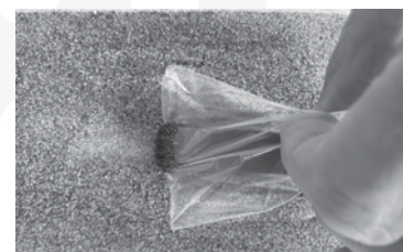
Magnet inside a plastic bag being rubbed through a sand sample and collecting ironsand.
