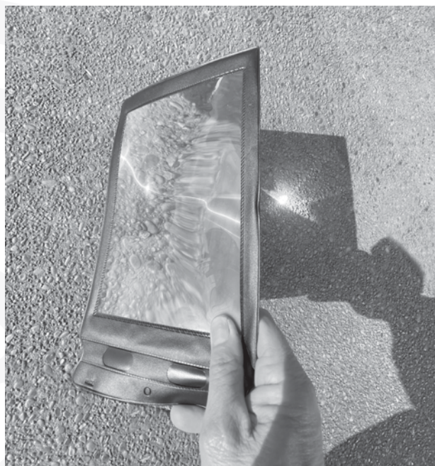
Directing the sun's rays through a Fresnel lens to make a small, bright spot on the ground.
