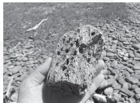
A pumice rock being jiggled up and down in the hand (called hefting) to feel how heavy it is. Feeling its weight and knowing its size gives an indication of its density.
