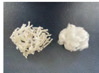
Natural fibres that can be mixed with paper pulp. Knitting wool (left, needs to be teased out first) and cotton wool.
